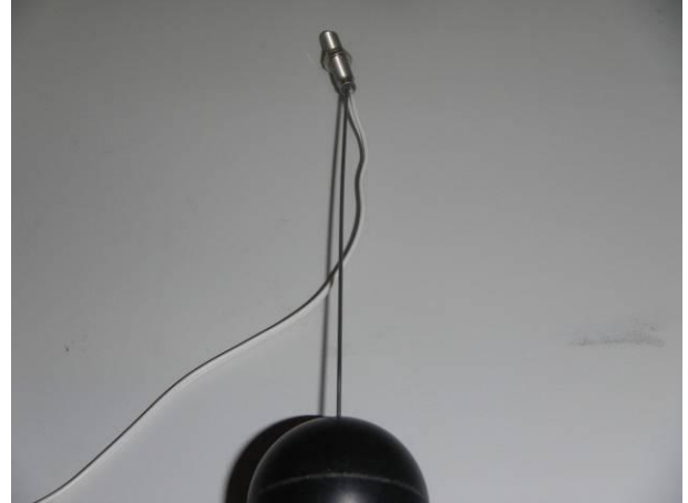
picture 2 MK11-1A66B-500W with test wire (Ø 1 mm, 1N) on the EUT (#4.1) during the protection against hazardous parts IP6X
