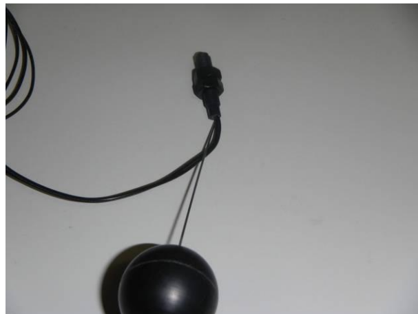
picture 2 MK11/M8-1A66B-500W with test wire (Ø 1 mm, 1N) on the EUT (#3.1) during the protection against hazardous parts IP6X
