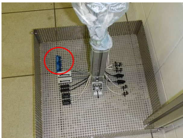
Picture 9 MK02/4-1A66C-500W - #1.1 and #1.2 mounted on a test frame after the immersion test IPX7
