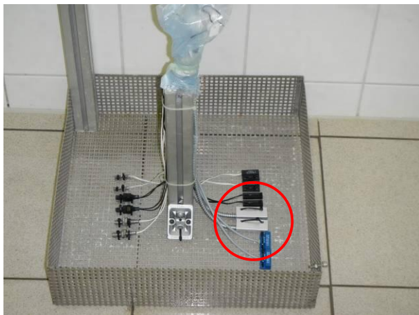
Picture 7 MK27-1A66B-500W - #7.1 and #7.2 mounted on a test frame after the immersion test IPX7
