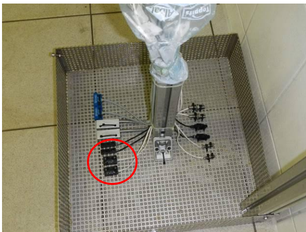
Picture 9 MK21P-1A66B-500W - #6.1 and #6.2 mounted on a test frame after the immersion test IPX7
