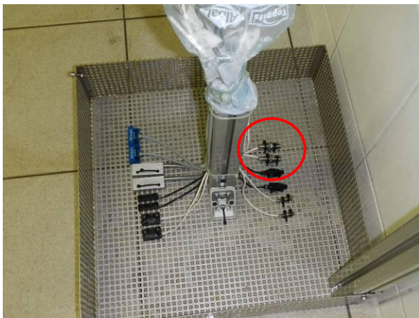
Picture 9 MK11/S8-1A66B-500W - #2.1 and #2.2 mounted on a test frame after the immersion test IPX7
