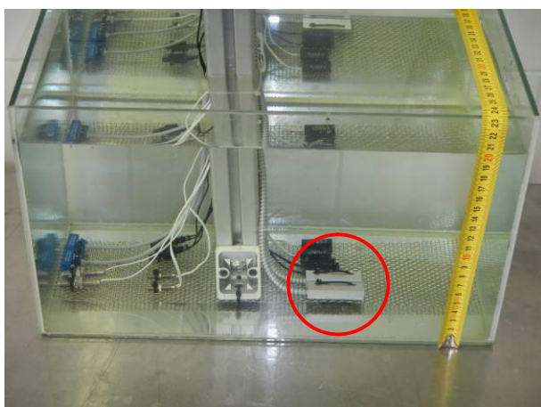
picture 5 MK27-1A66B-500W - #7.1 and #7.2 in the dip tank at a depth of 20 cm during the test IP6X (substitute test)
