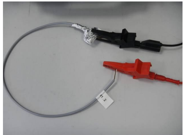
picture 4 MK02/4-1A66C-500W - #1.2 during the insulation resistance measurement before and after the tests IP6X and IPX7
