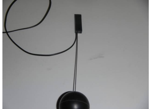
picture 2 MK26-1A66B-500W with test wire (Ø 1 mm, 1N) on the EUT (#5.1) during the protection against hazardous parts IP6X
