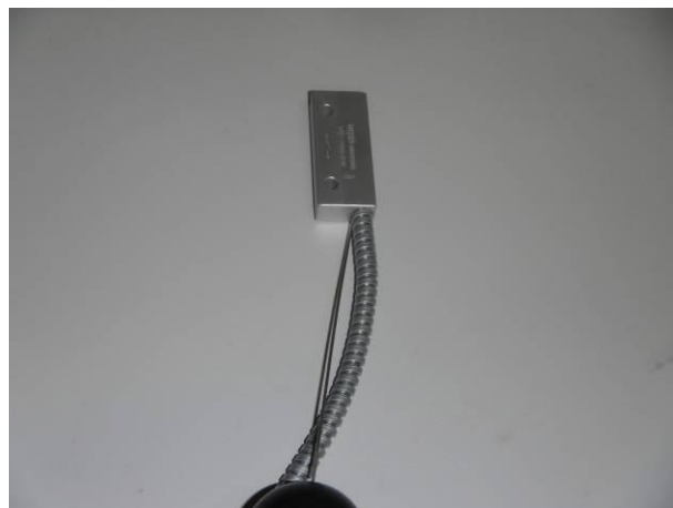
picture 2 MK27-1A66B-500W with test wire (Ø 1 mm, 1N) on the EUT (#7.1) during the protection against hazardous parts IP6X
