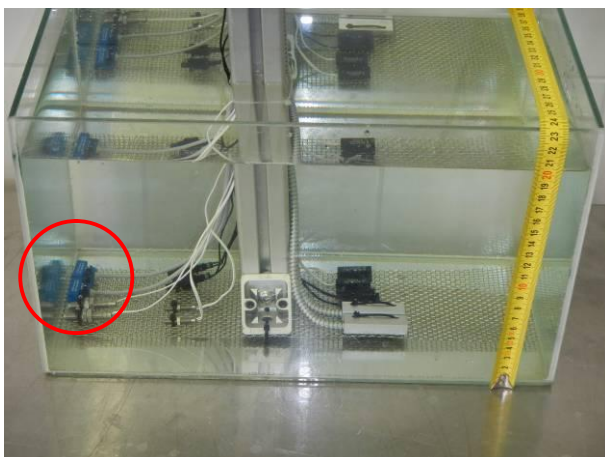
picture 5 MK02/4-1A66C-500W - #1.1 and #1.2 in the dip tank at a depth of 20 cm during the test IP6X (substitute test)
