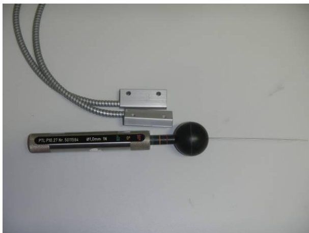
picture 1 MK27-1A66B-500W - #7.1 and #7.2 with test wire (Ø 1 mm, 1N) before the protection against hazardous parts IP6X
