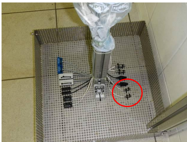
Picture 9 MK11-1A66B-500W - #4.1 and #4.2 mounted on a test frame after the immersion test IPX7
