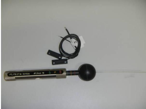
picture 1 MK26-1A66B-500W - #5.1 and #5.2 with test wire (Ø 1 mm, 1N) before the protection against hazardous parts IP6X
