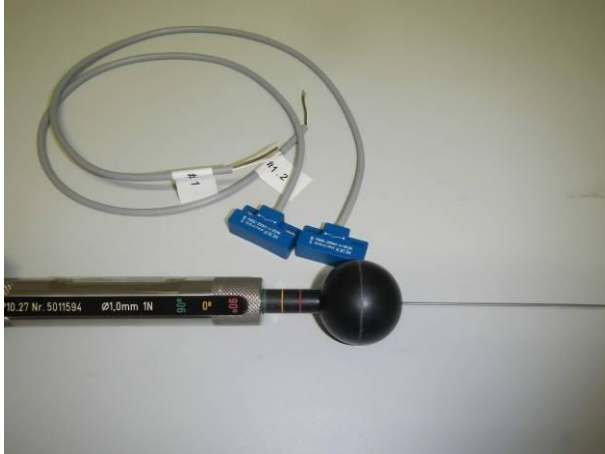
picture 1 MK02/4-1A66C-500W - #1.1 and #1.2 with test wire ( \varnothing 1 mm, 1N) before the protection against hazardous parts IP6X
