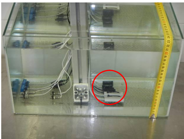
picture 5 MK21P-1A66B-500W - #6.1 and #6.2 in the dip tank at a depth of 20 cm during the test IP6X (substitute test)
