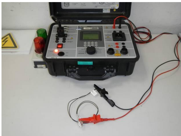
picture 3 MK11/M8-1A66B-500W - #3.1 during the insulation resistance measurement before and after the tests IP6X and IPX7
