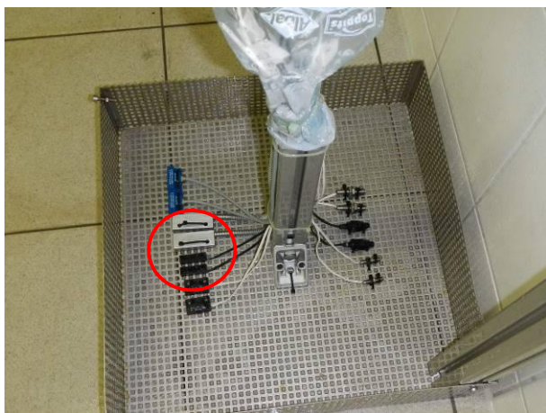
Picture 9 MK26-1A66B-500W - #5.1 and #5.2 mounted on a test frame after the immersion test IPX7
