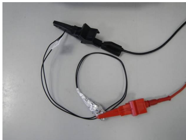
picture 4 MK11/M8-1A66B-500W - #3.2 during the insulation resistance measurement before and after the tests IP6X and IPX7
