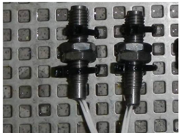
Picture 10 MK11/S8-1A66B-500W - #2.1 and #2.2 without visible external damage after the immersion test IPX7
