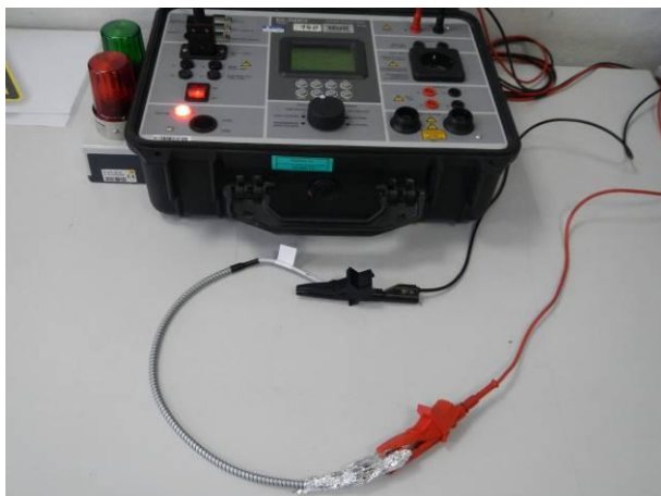
picture 3 MK27-1A66B-500W - #7.1 during the insulation resistance measurement before and after the tests IP6X and IPX7
