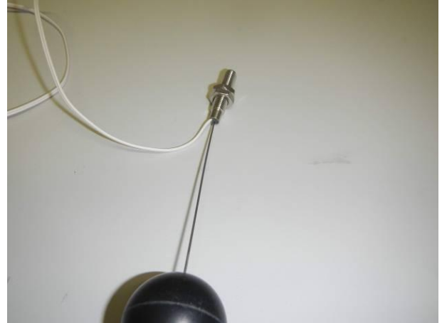
picture 2 MK11/S8-1A66B-500W with test wire (Ø 1 mm, 1N) on the EUT (#2.1) during the protection against hazardous parts IP6X
