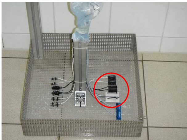
Picture 7 MK26-1A66B-500W - #5.1 and #5.2 mounted on a test frame after the immersion test IPX7
