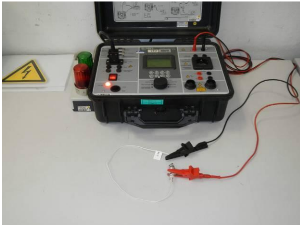
picture 3 MK11/S8-1A66B-500W - #2.1 during the insulation resistance measurement before and after the tests IP6X and IPX7
