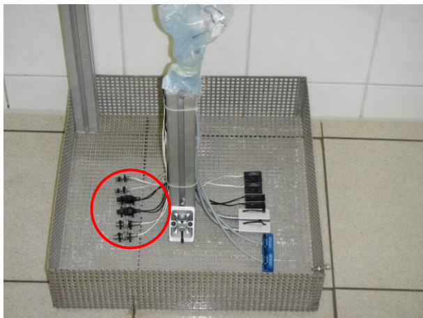
Picture 7 MK11/M8-1A66B-500W - #3.1 and #3.2 mounted on a test frame after the immersion test IPX7
