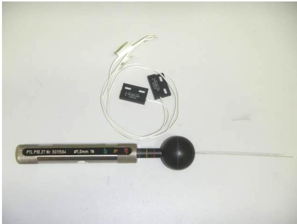
picture 1 MK21P-1A66B-500W - #6.1 and #6.2 with test wire (Ø 1 mm, 1N) before the protection against hazardous parts IP6X
