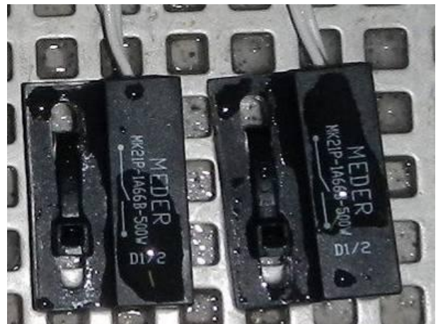
Picture 10 MK21P-1A66B-500W - #6.1 and #6.2 without visible external damage after the immersion test IPX7
