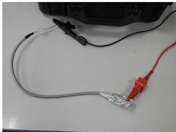
picture 4 MK27-1A66B-500W - #7.2 during the insulation resistance measurement before and after the tests IP6X and IPX7
