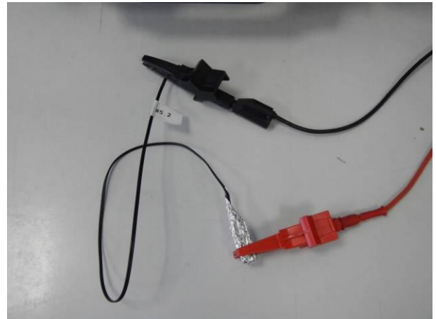
picture 4 MK26-1A66B-500W - #5.2 during the insulation resistance measurement before and after the tests IP6X and IPX7
