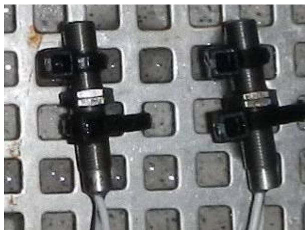
Picture 10 MK11-1A66B-500W - #4.1 and #4.2 without visible external damage after the immersion test IPX7
