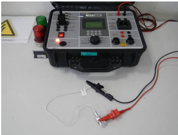
picture 3 MK21P-1A66B-500W - #6.1 during the insulation resistance measurement before and after the tests IP6X and IPX7
