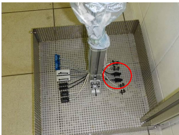
Picture 9 MK11/M8-1A66B-500W - #3.1 and #3.2 mounted on a test frame after the immersion test IPX7
