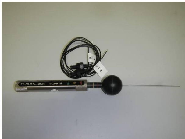
picture 1 MK11/M8-1A66B-500W - #3.1 and #3.2 with test wire (Ø 1 mm, 1N) before the protection against hazardous parts IP6X
