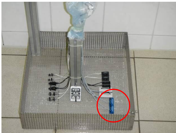
Picture 7 MK02/4-1A66C-500W - #1.1 and #1.2 mounted on a test frame after the immersion test IPX7
