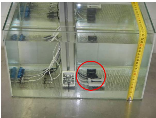
picture 5 MK26-1A66B-500W - #5.1 and #5.2 in the dip tank at a depth of 20 cm during the test IP6X (substitute test)
