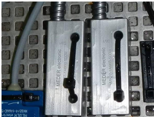
Picture 10 MK27-1A66B-500W - #7.1 and #7.2 without visible external damage after the immersion test IPX7
