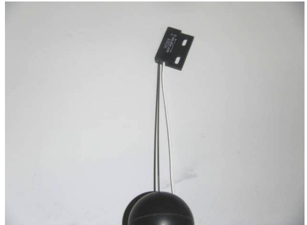
picture 2 MK21P-1A66B-500W with test wire (Ø 1 mm, 1N) on the EUT (#6.1) during the protection against hazardous parts IP6X
