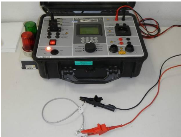
picture 3 MK02/4-1A66C-500W - #1.1 during the insulation resistance measurement before and after the tests IP6X and IPX7
