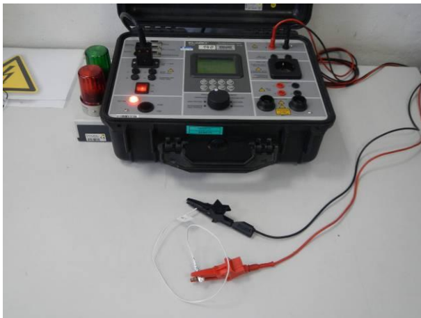
picture 3 MK11-1A66B-500W - #4.1 during the insulation resistance measurement before and after the tests IP6X and IPX7
