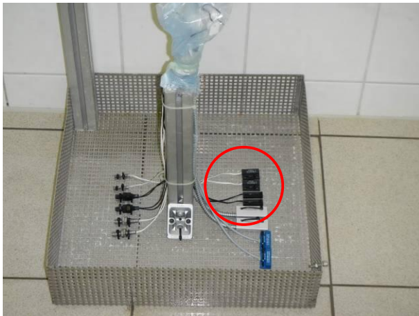
Picture 7 MK21P-1A66B-500W - #6.1 and #6.2 mounted on a test frame after the immersion test IPX7
