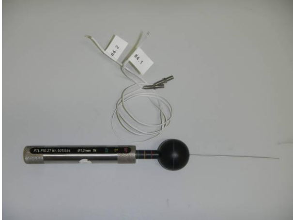
picture 1 MK11-1A66B-500W - #4.1 and #4.2 with test wire (Ø 1 mm, 1N) before the protection against hazardous parts IP6X
