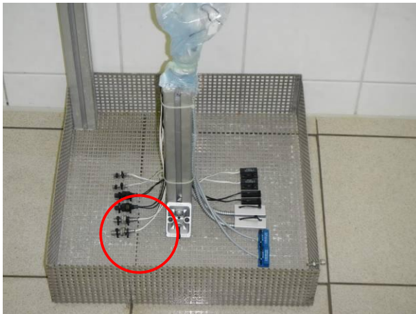
Picture 7 MK11/S8-1A66B-500W - #2.1 and #2.2 mounted on a test frame after the immersion test IPX7
