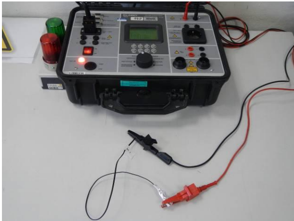
picture 3 MK26-1A66B-500W - #5.1 during the insulation resistance measurement before and after the tests IP6X and IPX7
