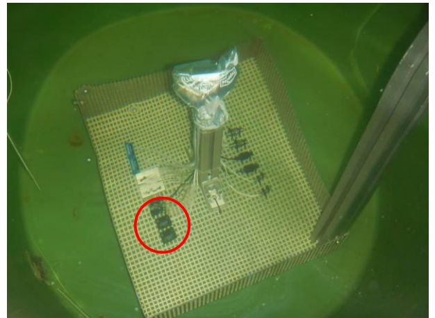
Picture 8 MK21P-1A66B-500W - #6.1 and #6.2 in the dip tank at a depth of 1 m after the immersion test IPX7
