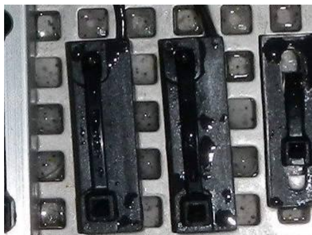
Picture 10 MK26-1A66B-500W - #5.1 and #5.2 without visible external damage after the immersion test IPX7
