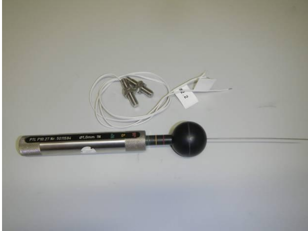
picture 1 MK11/S8-1A66B-500W - #2.1 and #2.2 with test wire (Ø 1 mm, 1N) before the protection against hazardous parts IP6X
