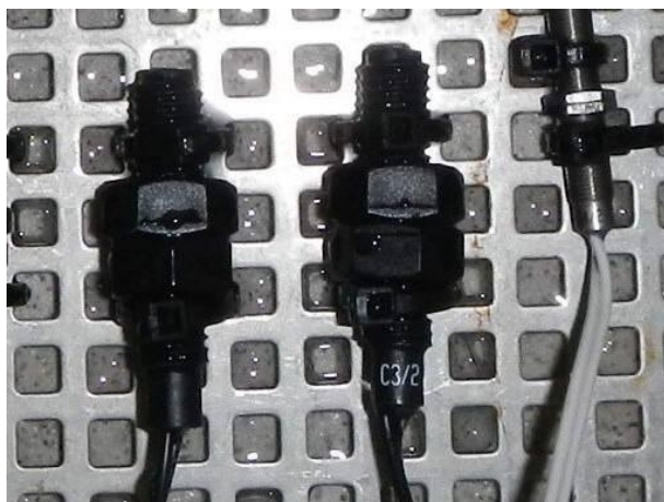
Picture 10 MK11/M8-1A66B-500W - #3.1 and #3.2 without visible external damage after the immersion test IPX7
