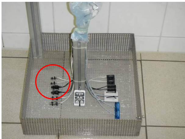
Picture 7 MK11-1A66B-500W - #4.1 and #4.2 mounted on a test frame after the immersion test IPX7
