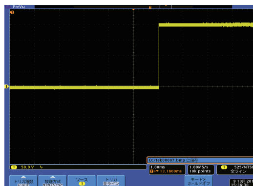
Example of voltage waveform when 200V is applied
