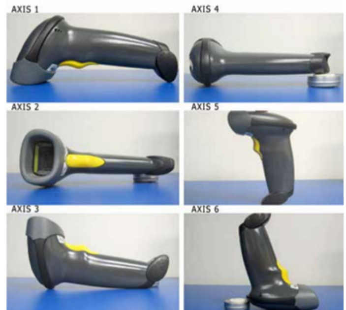
Figure 4 Electronic barcode scanner drop test axes.
